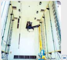
**34.** Test chamber for quickaging of high voltage isolators: temp., humidity, sun light (UV), rain, salt fog. Useful capacity: 700 m³ (courtesy of EDF France).
