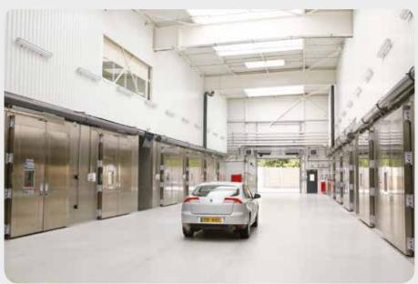
44. Airbag test chamber equipped with a high speed opening and closing door system for quick deployment (7 seconds approx.) of the specimen on a dedicated trolley.
