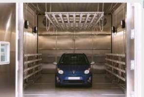
29. Standard Discovery My chamber equipped with sun simulation system.30. Solar radiation system provided with a special lamp
